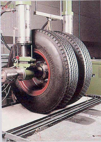
Wheel load testing at the TU Munich - test bench
