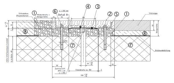
Figure 1: Standard cross section of the FPEJ system HEWA JOINT HJ30 (representative for the systems without stabilizing elements)
