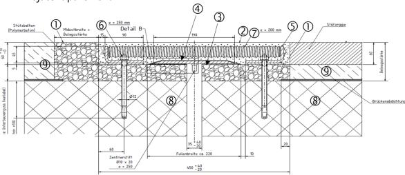
Figure 2: Standard cross section of the FPEJ system HEWA JOINT HJ60 (representative for the systems with stabilizing elements)
